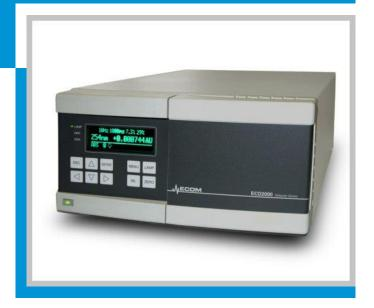
Cell could be easily removed from the front of the unit. Three selectable flow cells **AD02**, **AD05** and **AD10** with optical path length 2.4, 5 and 10 mm. AD05 cell is included as component of the detector. Other cells on request.
