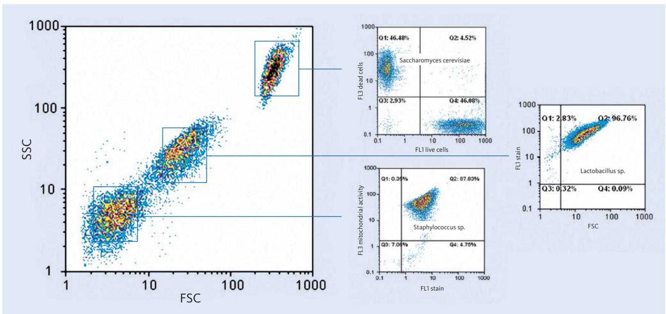
**Figure 2** Separation of differently sized organisms during a single measurement in a scatter plot: *Staphylococcus sp.* – *Lactobacillus sp.* – *Saccharomyces cerevisiae*. The subsequent analysis comprised mitochondrial activity measurement of *Staphylococcus*, DNA staining of *Lactobacillus*, and viability measurement of *Saccharomyces*.
