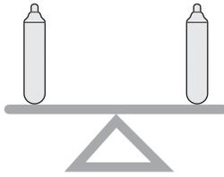
2. Load the filled containers symmetrically into the rotor. (Refer to TUBES AND BOTTLES on page 7 for information about containers.) If fewer than twelve tubes are being run, they must be arranged symmetrically in the rotor (see Figure 1). Opposing tubes must be filled to the same level with liquid of the same density.
