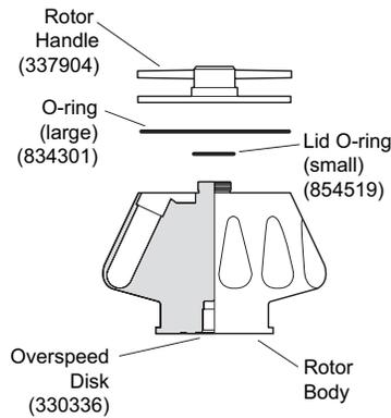
The Type 50.2 Ti, rated for 50 000 rpm, is a fixed angle rotor designed to centrifuge up to twelve tubes at a 24-degree angle to the axis of rotation. Used in Beckman Coulter class H, R, and S preparative ultracentrifuges, the rotor develops centrifugal forces sufficient for the differential separation of particles, and for equilibrium sedimentation of particles such as DNA and viruses. Up to 468 mL of gradient and sample volume can be centrifuged per run.
