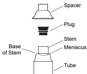
OptiSeal tubes come with plastic plugs and can be quickly and easily prepared for use. With the tube spacer in place, the *g* force during centrifugation ensures a tight, reliable seal that protects your samples.
