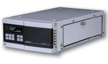
Peltier heating/cooling column oven (0-80°C) with a big compartment room can accommodate up to 3 columns with length up to 25 cm. Unit is controlled via keypad, RS232orLANInterface.
