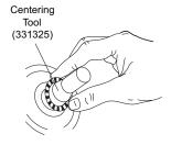
• Regularly inspect the overspeed disk. If it is scratched, damaged, or missing, replace it. *Rotors and Tubes* contains instructions for replacing the overspeed disk.
